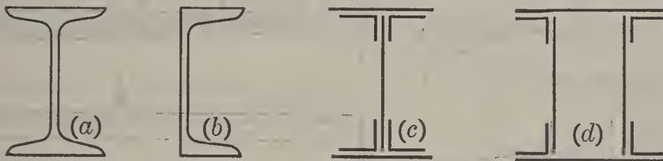
FIG. 110.—Sections having large values of \frac{I}{c}
